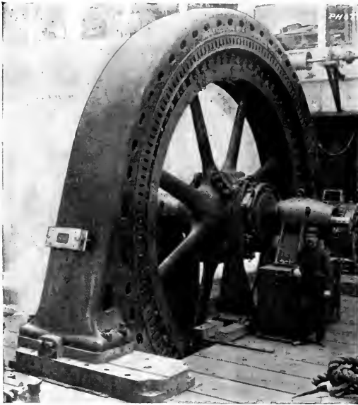
FIG. 4.—MODERN ENGINE TYPE OF REVOLVING-FIELD ALTERNATOR, 2,000 KW.
